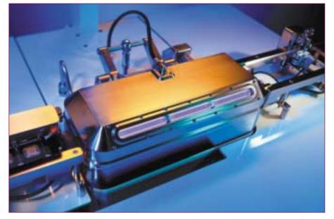
This single strip, compact plasma chamber processes BGA-type substrates with argon plasma.
